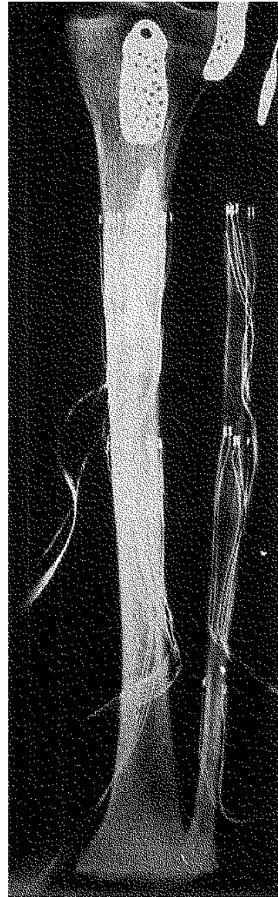
Fig. 2. — Radiograph of the tibiofibular frame with strain gauges.
