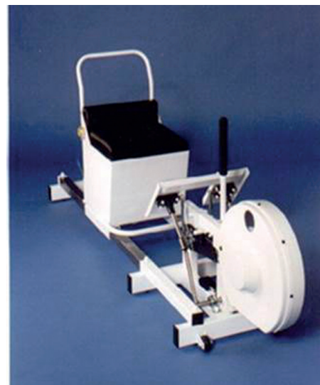
Figure 3. — The lab set-up with the Leg Extensor Power Rig
