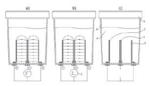
Fig. 2. — Drawing of the electric field distribution of the three different electric models: a) Plate negatively charged, b) Plate positively charged, c) Control plate without current). Detail of numbers: 1- Plate Under Test or circular metal plate; 2- Lateral L-plates; 3- pulse wave generator; 4- liquid medium with bacteria; 5- container for urine sample; 6- tight cover that keeps sealed the recipient.
