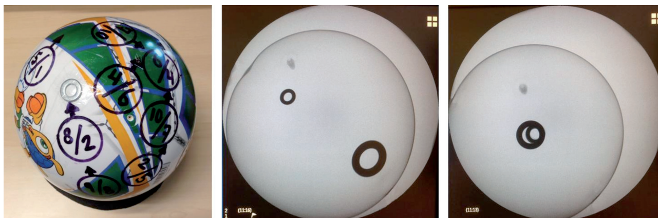
Fig. 1. — Macroscopic and fluoroscopic images of the soccer ball with A. two random series of predefined positions and B. washers not aligned and C. washers aligned
