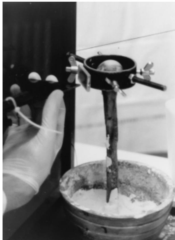
Fig. 3. — Calibration of the laser reflexion to measure relative displacement of the humeral head.
