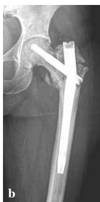
Fig. 3b. — Failure of the titanium trochanteric Gamma nail on the level of the aperture for the lag screw.
