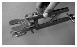
*Fig. 1.* — Spreader tool prototype – the lower plate rests on the tibial cut, the upper plate swivels and lifts the femoral condyles, as the soft tissues are put under tension by turning the screw.
